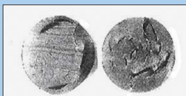
● Fig. 1. Internal cracks in the O-ring.
