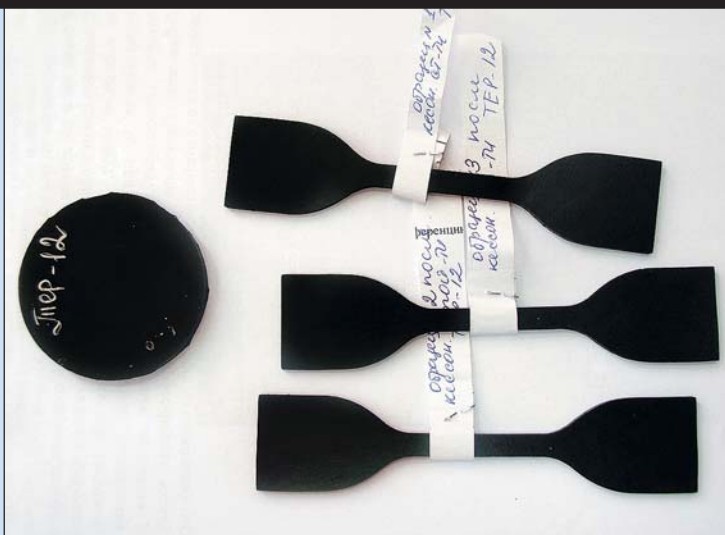
● Fig. 2b. A Therban-based rubber compound resistant to ED. After testing this sample retained its functional properties and dimensions.
